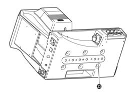
**@**Screw Holes for Mounting Tripod
